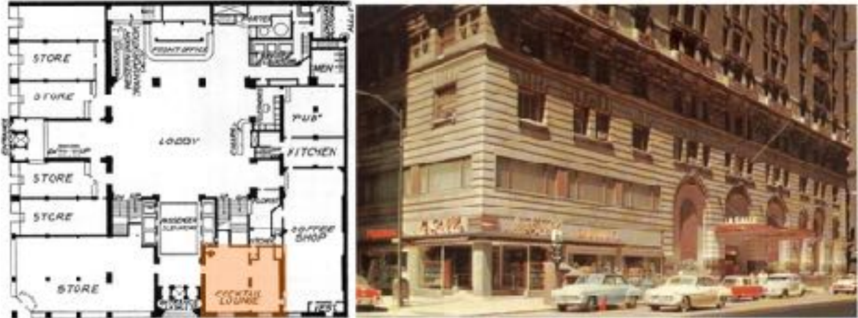
Above: Ground floor plan of Hotel LaSalle. Fire started at point X, spread throughout cocktail lounge, then through unprotected door into lobby and up the open stairs and pierced elevator shafts.
